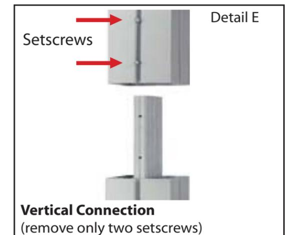
When vertical extrusions are packed in portable cases rather than crates or tubs, they must be broken down into smaller sections which then require assembly.
